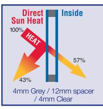
Chevron Insulated Glass Unit using toned glass can reduce heat gain by 27%.
