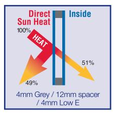
Chevron Low E Insulated Glass Unit using Low E glass on the inside pane can reduce heat gain by 33%.
